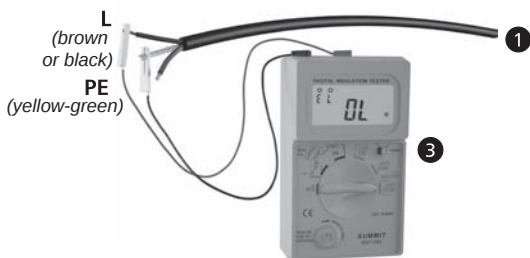
Insulation resistance measurement
